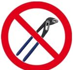
Warning: Don't use pipe wrenches or pliers to screw nozzles and accessories. Use the right wrenches for each product and if necessary request ILMAP the appropriate equipment.
