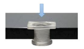
Check holes in the plate! Hole for sleeve MP range 31,5 - 32,0 mm - 15/16"W range 37,0 - 37,5 mm - 11/4"W
