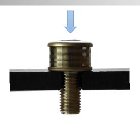
Check holes in the plate! Make sure the hole is suitable for the Nozzle's thread
