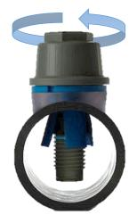
Check the assembly! The Nozzle will not have to move and saddle have to join perfectly with the pipe
